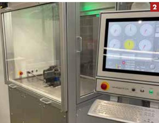
**2** With our new "servo motor driven" test bench (from end 2022), 45kW, 315 bar and 80 l/min, valves are adjusted even more comprehensively and accurately.
